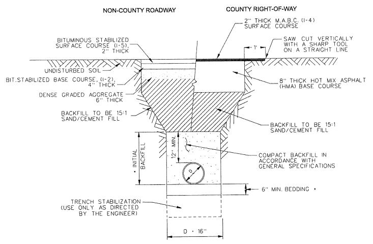
• INITIAL BACKFILL AND BEDDING MATERIAL SHALL BE SOIL AGGREGATE DESIGNATION I-8 CONFORMING TO THE REQUIREMENTS OF ARTICLE 901.09 TABLE 901-2 OF THE STANDARD SPECIFICATIONS, 1983 SUPPLEMENT, OR STONE CRUSHINGS TO CONFORM WITH AASHTO DESIGNATION M-43-54 (1974) (ASTM DESIGNATION D448-54), SIZE NO. 8, 1/8" TO 3/8" (2.36 mm TO 9.25 mm) CLEAN, FREE FLOWING AND SHALL MEET ALL ASTM C-33 FOR QUALITY AND SOUNDNESS.
